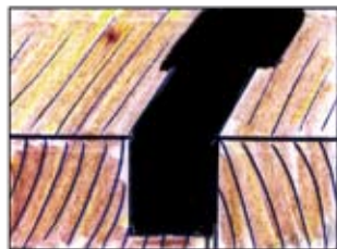
7. When cured sand off top as required
