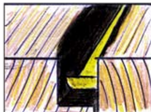
4. Apply Breaker Tape if required.
